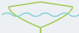
A v-shaped hull decreases the surface area of water in contact with the ship. This decreases the buoyancy force acting on the ship. It also reduces the friction, or water resistance, so the ship can go faster through the water. A v-shaped hull causes the bow of the ship to pierce through the waves rather than go over them so increases stability in rough water. Navy ships have a v-shaped hull.
