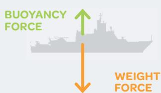
The weight force is greater than the buoyancy force showing that the ship is moving in the downwards direction.
